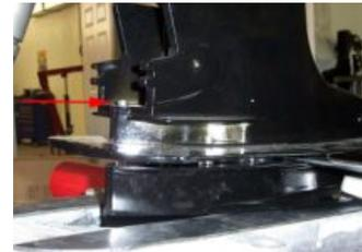
**2.9** Install the front nut and the trim tab. Spin the prop after the trim tab is installed to check for clearance.
