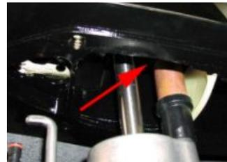
**2.3** Install the brass shift shaft into the upper housing. Insert the brass piece, then install the washer, and then the cotter pin.
