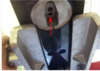
**1.2** Remove the bolt that is under the trim tab. Use the 5/16" Allen key.
