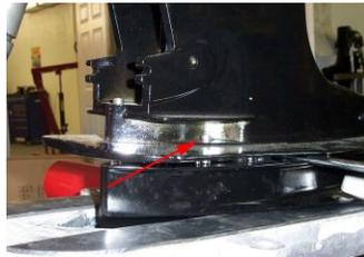
**2.7** Now you can start to install the hardware. First install the two side nuts. The drive has to be separated to install them, so you should still have the screwdriver in between the halves. Once both of the nuts are started, you can then pull the screwdriver out and tighten the nuts.
